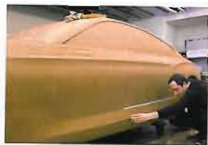
Clay model of a new car design
